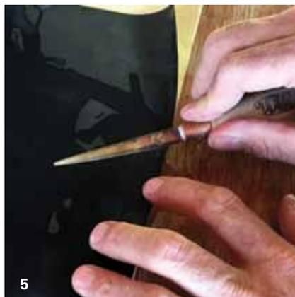
5 Use wet/dry sandpaper on a flat, smooth surface when sharpening long, flat blades.
