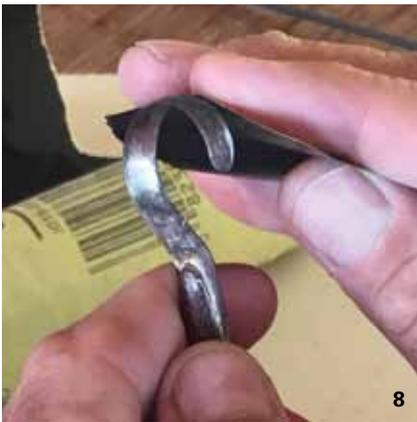
Use wet/dry sandpaper to remove burrs from the back of newly sharpened edges.
