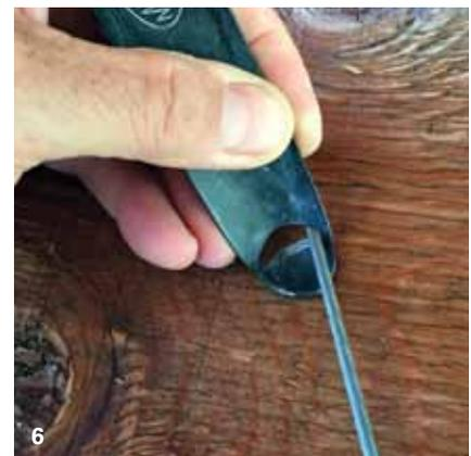
6 Use even pressure while simultaneously pushing the file forward and side to side.
