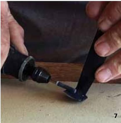
Use a light touch with a Dremel/rotary tool with a diamond burr sharpening bit.
